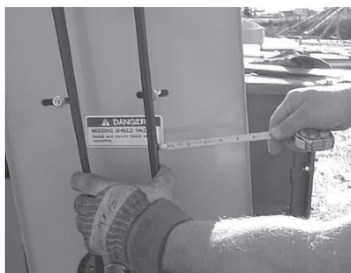
Push on center span of belt 5-10 lbs.
