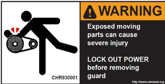
To be placed on removable guards to warn that operation of the machinery with guards removed would expose chains, belts, gears, shafts, pulleys, couplings, etc. which create hazards.
